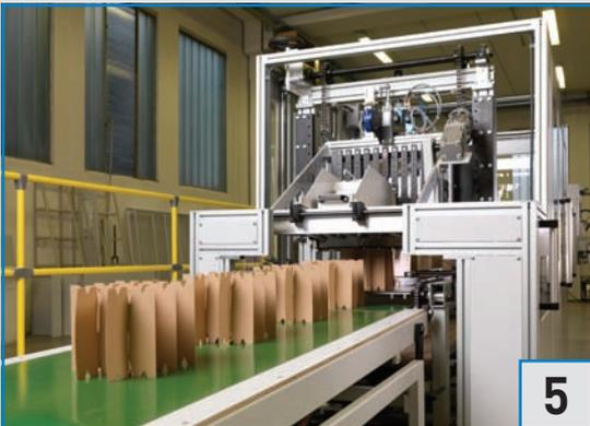
Assembled partitions are then delivered out of the machine by means of a belt conveyor, to be collected by hand or fed automatically in the **COLLAPSER (OPT)** closing and stacking device.
