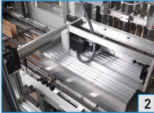
Longitudinal elements are to be fed vertically onto the conveyor belt, inside the guiding channels. Standard machine is endowed with 9 guiding channels, more on request. Channels feeding operation it's done by a movable carriage.
