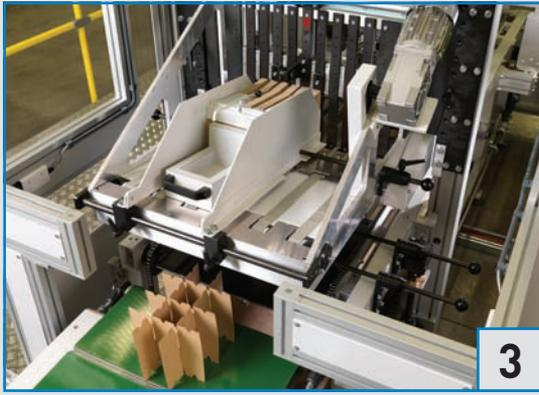
Cross dividers feeder is installed on the top of the interlocking area, in the middle of the machine. Elements are kept upright by a pressure system and moved to the injection area by means of belts.
