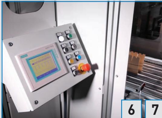
Machine is controlled and operated from the touch screen panel, installed on the machine closer to the operator side. From this HMI the operator processes and saves the data related to the different partitions like number of cuts in longitudinal element, motors speed, injection timing, etc.
